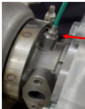
Tighten speed sensor to 15.0 – 17.0 Nm
