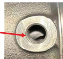
Above pictures show bearing spacer hole not aligned with center housing hole.
