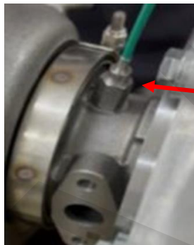
Tighten speed sensor to 15.0 – 17.0 Nm
